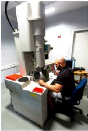
Figure 2.23 A Transmission Electron Microscope. The electron gun is at the top of the central column, and the magnetic lenses are within the column. The image on the fluorescent screen is also viewed on a computer monitor. © McGraw Hill Education
